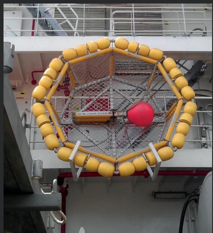
Our Dacon Rescue Basket is ideal for mass rescue situations. The basket is operated by a deck crane and while in use the basket is lowered into the water. During operation, the basket has a low floating point which makes for an easy entry. The yellow bumpers will protect both the individual and the vessel itself from damage in rough seas. The equipment is fit with an aluminium construction which makes it strong and durable.
